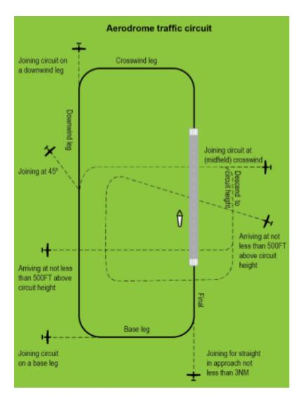
Figure 5 Aerodrome standard traffic circuit, showing arrival and joining procedures
