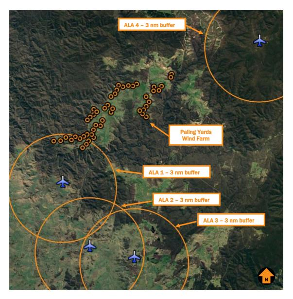
Figure 16 ALAs with 3 nm buffer
