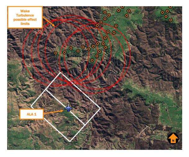
Figure 20 Wake turbulence possible effects in the northern circuit at ALA 1
